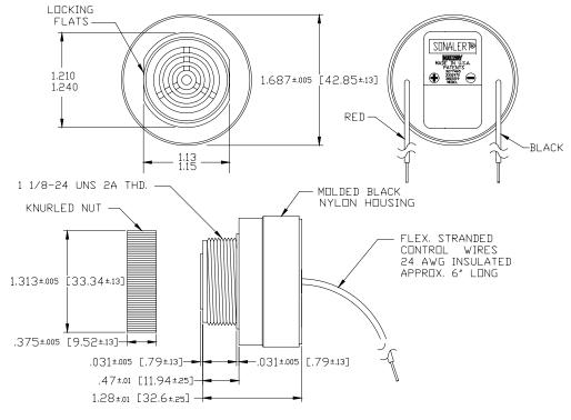
NOTE: MOUNTING- REMOVE BLACK PLASTIC NUT AND INSERT THREADED FRONT THROUGH 1.25" HOLE PUNCHED IN PANEL, IF ORIENTATION IS NEEDED, NOTE LOCKING FLATS ON DRAWING. SCREW NUT BACK ON. DO NOT OVERTIGHTEN.
